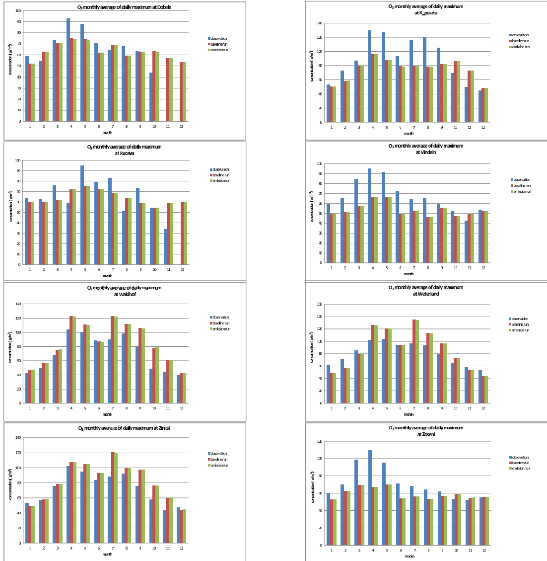
Figure 9: Monthly mean maximum ozone concentration ( \mu\text{g m}^{-3} ) at eight measurement stations (table 5) along with modelled values from the baseline and emission simulations.
