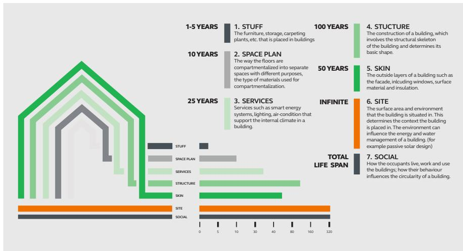
Figure 1 The 7 layers of a building. Building model consisting of six material layers (after Steward Brand (1994) and David Bergman (2011) and a seventh social layer. Each layer has an own life cycle, with different lifespans.
