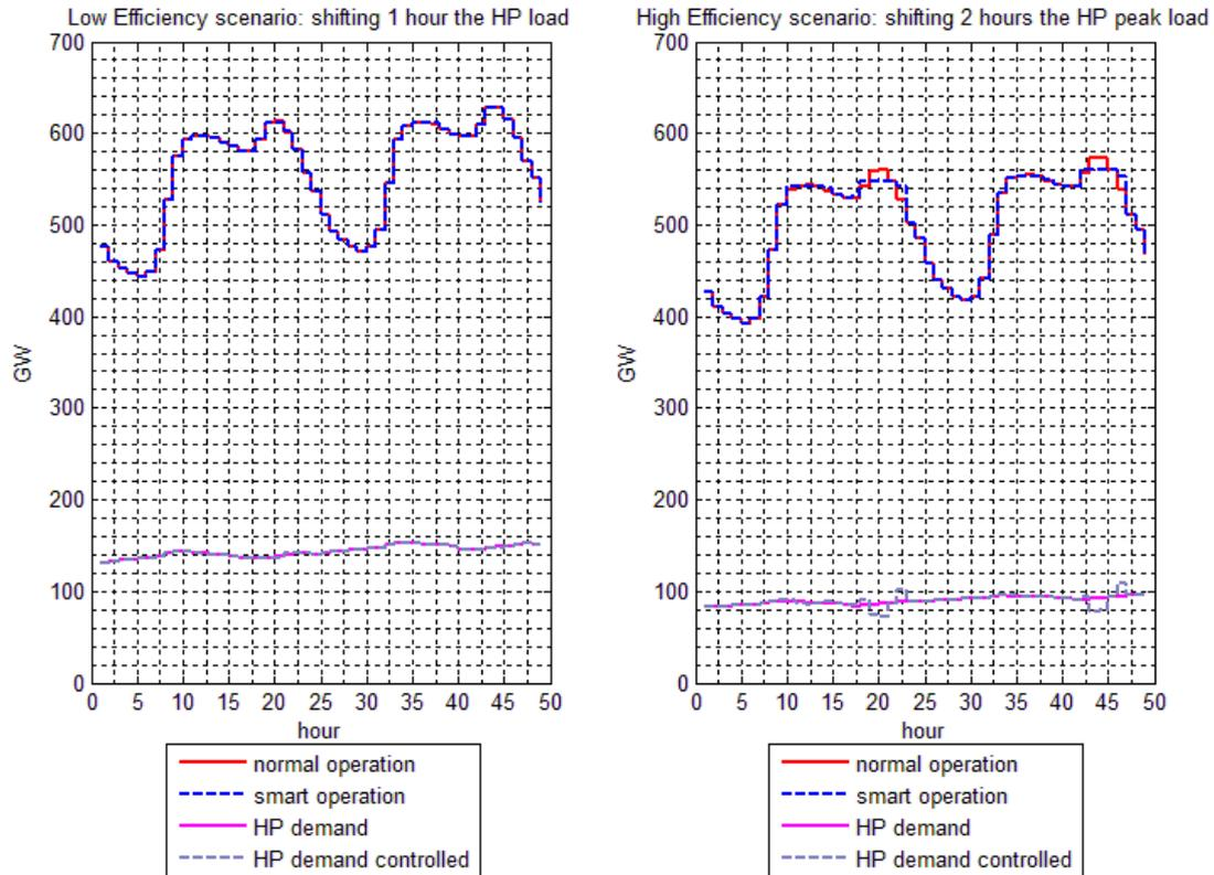
Figure 7: Daily load shape of the estimated EU electricity demand of buildings and the heat pump electricity consumption: Low Efficiency scenario with the option of shifting heat pump consumption by one hour (left) – High Efficiency scenario with the option of shifting heat pump consumption by two hours (right)
