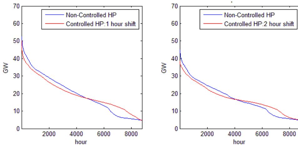
**Figure 10** Load duration curve of each scenario showing the total impact of each heat demand flexibility option on the German power system. (Left) low efficiency scenario. (Right) high efficiency scenario.
